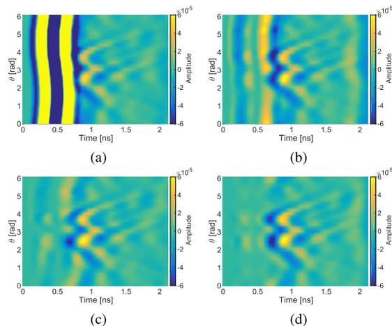
**Fig. 5** Signal subtraction results in CASE 2. (a) Original signal. Clutter eliminated signals by the method I (b), the method II (c) and the proposed method (d).
