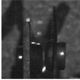
**Fig. 4** Arc behavior image almost immediately before extinction with the applied magnetic field of  $B = 120\text{mT}$  but no magnetic blowing at 20V-7A (Note this image was captured with the opening speed of 10mm/s).
