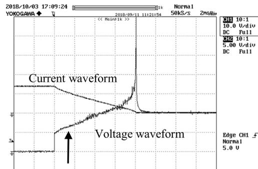
Fig. 2 Exemplary voltage/current waveforms with magnetic field of  $B = 120\text{mT}$  at 20V-7A with the opening speed of 50mm/s.
