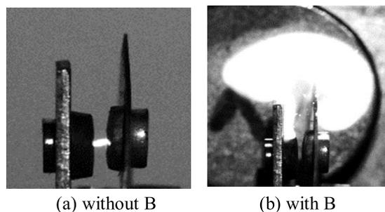
Fig. 3 Exemplary arc behavior images almost immediately before extinction without/with the applied magnetic field of  $B = 120\text{mT}$  at 14V-12A with the opening speed of 50mm/s.
