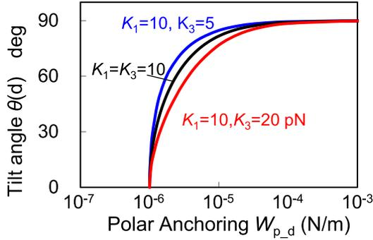
Fig. 2 Anchoring strength of  $W_{p,d}$  vs. tilt angle  $\theta(d)$ .  $W_{p,0}$  is infinite.
