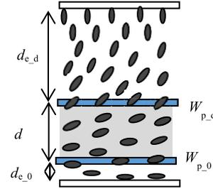
Fig. 5 Schematic model of HAN cell with finite anchoring surfaces in the case of  $W_{p,d} < W_{p,0}$  ( $d_{e,d} > d_{e,0}$ ).
