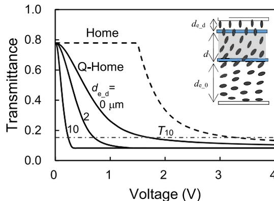
**Fig. 7** Transmittance as a function of applied voltage in GH mode Q-Home cells with weak anchoring substrates of  $W_{p,d} > W_{p,0}$ .
