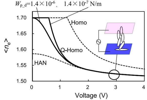
Fig. 4 Effective extraordinary refractive index vs. applied voltage in Q-Homo, HAN and Homo cells.
