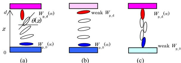
**Fig. 1** Schematic model of LC director distribution in (a) HAN, (b) quasi homogeneous and (c) quasi homeotropic cells.
