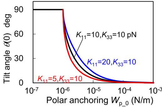
Fig. 3 Anchoring strength of  $W_{p,0}$  vs. tilt angle  $\theta(d)$ .  $W_{p,d}$  is infinite.
