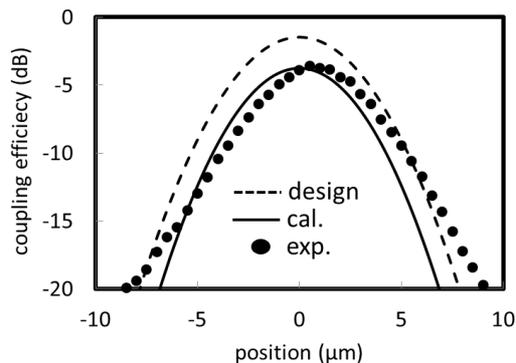
**Fig. 5** Measured and calculated coupling efficiency between the LISEL and SMF with respect to the SMF position.
