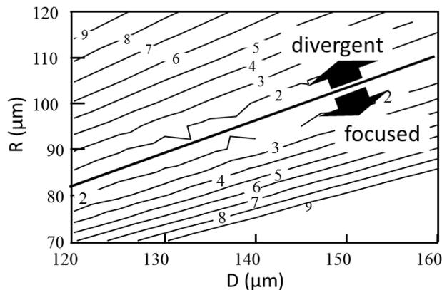
Fig. 2 Contour plots of calculated angle of far-filed pattern from LISEL.
