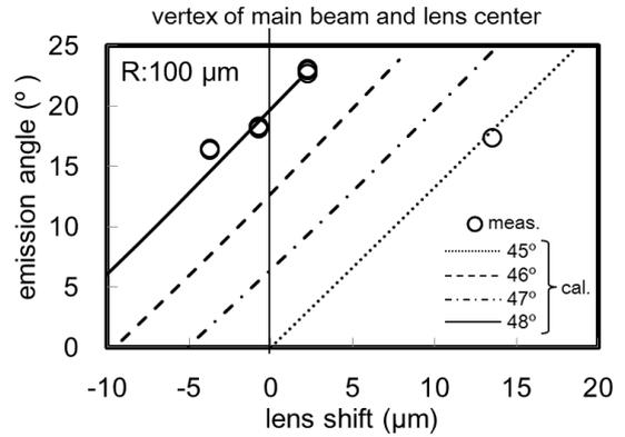
**Fig. 10** Emission angle vs lens shift under various mirror angle.
