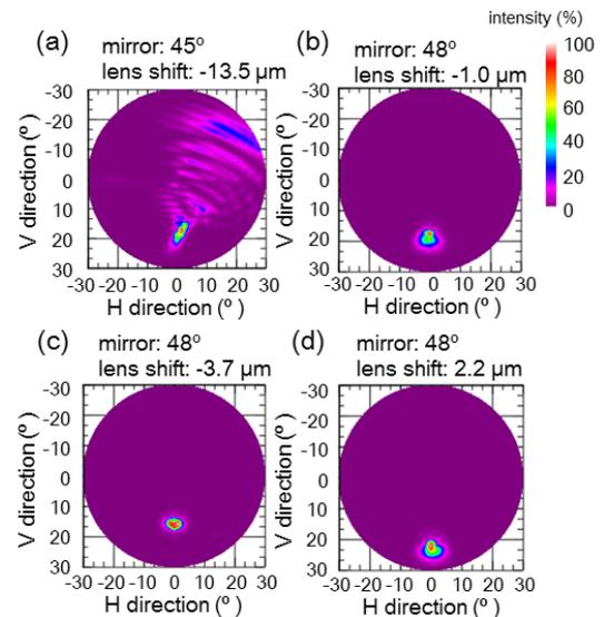
**Fig. 11** Measured far-field patterns, (a) mirror angle of  $45^\circ$ , (b), (c), and (d) mirror angle of  $48^\circ$ .
