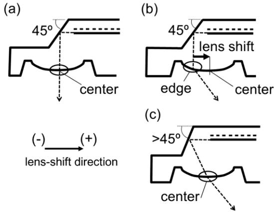
**Fig. 8** Principal of emission-beam control. (a) standard position (vertical emission), (b) angled beam with lens shift, and (c) angled beam with lens shift and mirror angle shift from  $45^\circ$ .
