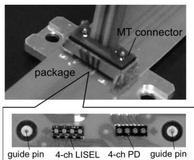
**Fig. 6** Photograph of the fabricated OSA. Enlarge shows the 4ch-LISEL array and PD array bonded on the package.
