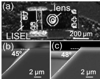
**Fig. 9** Fabricated LISEL for SiP platform. (a) Top view of the device with integrated lens, (b) and (c) cross-section of SEM images of  $45^\circ$  and  $48^\circ$  mirror, respectively.
