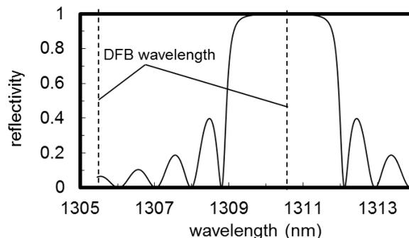
Fig. 14 Theoretical calculation of DBR reflective and two lasing wavelengths of DFB laser with uniform grating.
