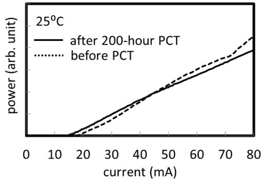
**Fig. 16** Measured light-current characteristics of facet-free DFB laser before/after PCT.
