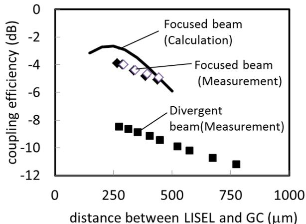
Fig. 12 Coupling loss from LISEL to GC.
