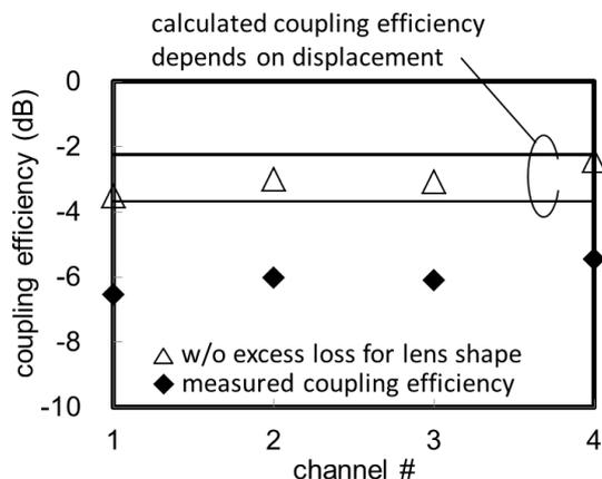
**Fig. 7** Coupling efficiency between LISEL array and SMF array by using passive optical alignment technique.
