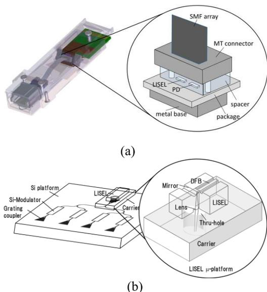
**Fig. 3** Conceptual structure of cost-effective OSA with LISEL. (a) Image of optical module and OSA consisting of passively aligned LISEL array and SMF array. (b) OSA consisting of silicon platform integrated with LISEL  $\mu$ -platform as light source.
