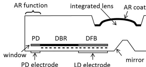
Fig. 13 Schematic structure of facet-free DFB laser based on the LISEL.
