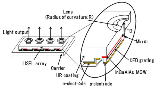
Fig. 1 Schematic structure of 4-ch LISEL array. Enlarge view shows cross section of the DFB laser stripe.
