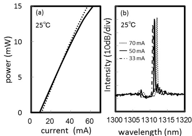
Fig. 15 Lasing characteristics of the DFB laser with facet-free structure, (a) light current curve, and (b) lasing spectra at bias current of 33, 50, 70 mA.
