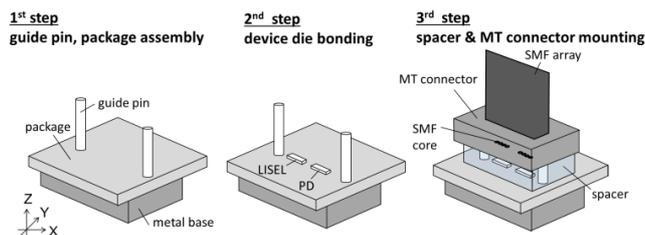
**Fig. 4** Assemble process of OSA consists of 4-ch LISEL array and SMF array (MT connector).
