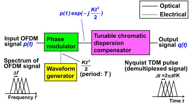
Fig. 1 Schematic and operating principle of tunable optical OFDM demultiplexer.
