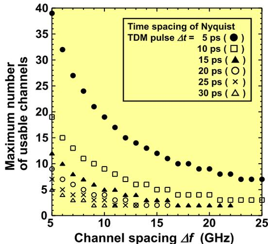
Fig. 3 Maximum number of usable channels versus channel spacing with regard to OFDM sub-carriers.
