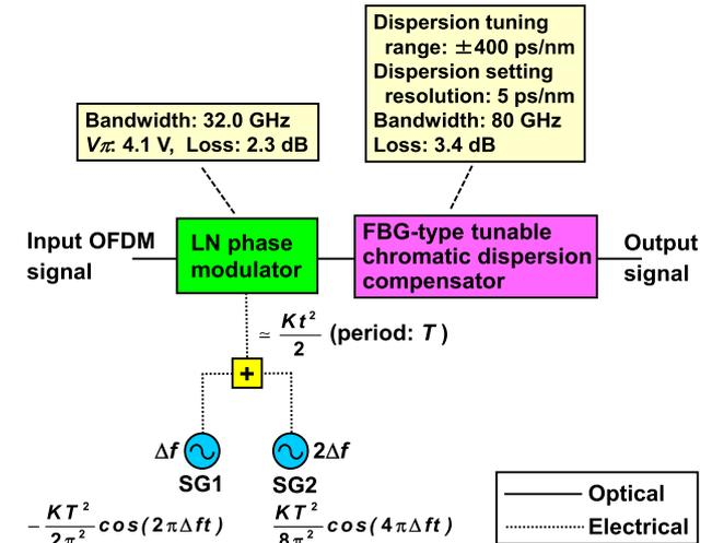
Fig. 4 Specific configuration of tunable optical OFDM demultiplexer.
