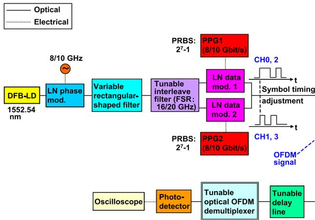
Fig. 5 Experimental set-up to evaluate tunable OFDM demultiplexer.
