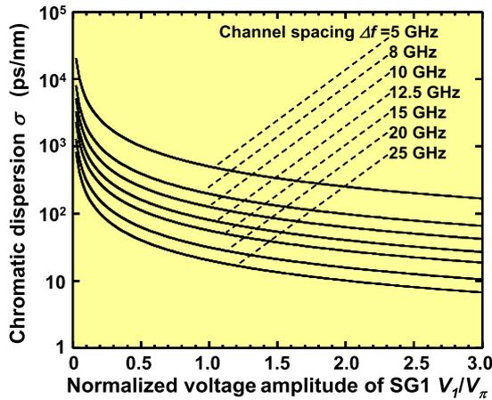
Fig. 2 Relation between chromatic dispersion  $\sigma$  and SG1 voltage amplitude normalized by modulator half-wave voltage  $V_1/V_\pi$ .
