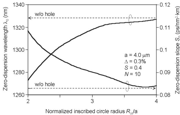
**Fig. 8** Calculated zero-dispersion wavelength  $\lambda_0$  and zero-dispersion slope  $S_0$  as a function of normalized inscribed circle radius  $R_{in}/a$ .
