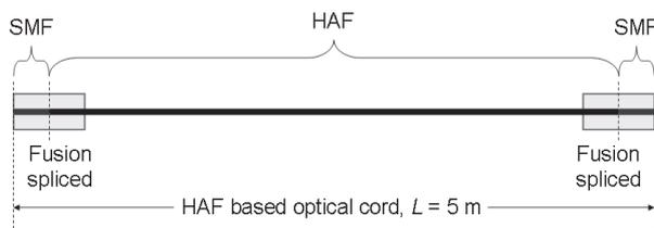
**Fig. 9** Schematic image of HAF based optical cord.
