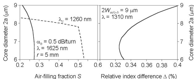
**Fig. 7** Optimum design conditions for HAF with desired MFD, bending-loss and cutoff wavelength characteristics.
