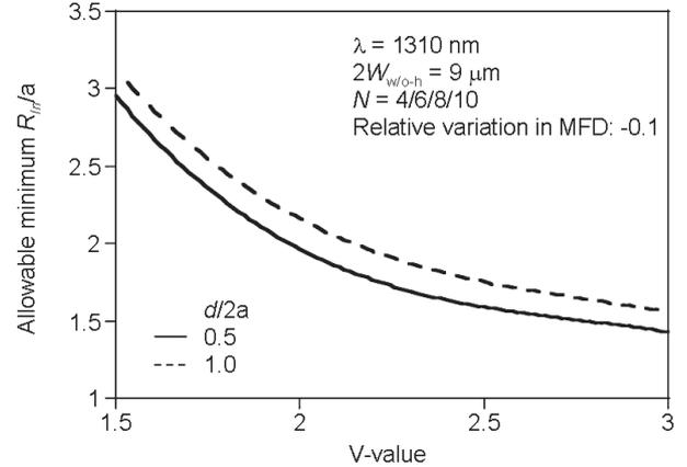
**Fig. 3** Allowable minimum  $R_{In}/a$  as a function of  $V$  value when the relative variation in MFD was set at  $-0.1$  at 1310 nm.
