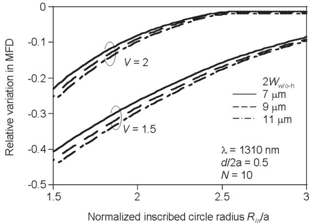
**Fig. 2** Relative variation in MFD as a function of normalized inscribed circle radius  $R_{In}/a$  calculated at 1310 nm.
