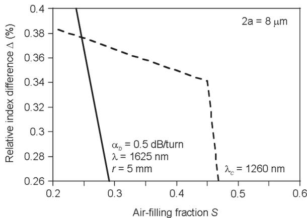
**Fig. 6** Calculated relationship between air filling fraction  $S$  and relative index difference  $\Delta$  when we set  $2a$  at  $8\ \mu\text{m}$ .
