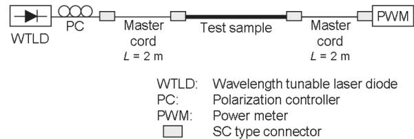
**Fig. 10** Experimental setup for measuring MPI.
