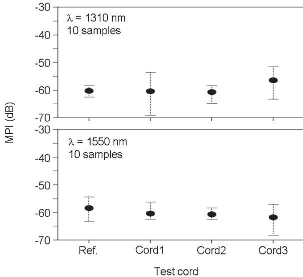
**Fig. 11** MPI of HAF based optical cord measured at 1310nm (upper) and at 1550 nm (lower).
