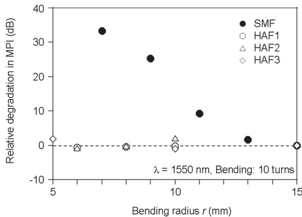
**Fig. 12** Relative variation in MPI as a function of bending radius  $r$ .
