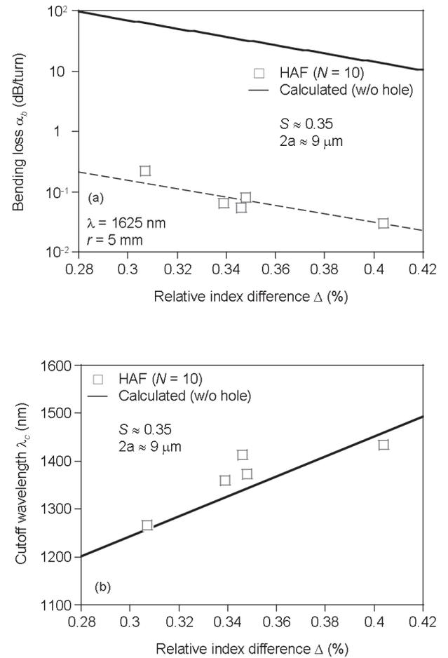
**Fig. 5** Relative index difference  $\Delta$  dependences of (a) bending-loss  $\alpha_b$  and (b) cutoff wavelength  $\lambda_c$ .
