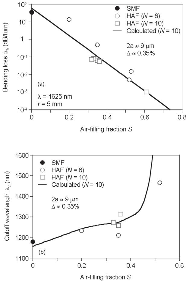
**Fig. 4** Air filling fraction  $S$  dependences of (a) bending loss  $\alpha_b$  and (b) cutoff wavelength  $\lambda_c$ .
