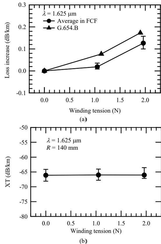
Fig. 6 Winding tension dependence of (a) the loss increase and (b) the inter-core XT at a wavelength of 1.625  $\mu$ m
