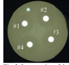
Fig. 3 Cross section of the fabricated FCF
