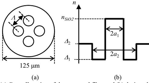
Fig. 1 (a) Core allocation of the proposed fiber and (b) designed index profile
