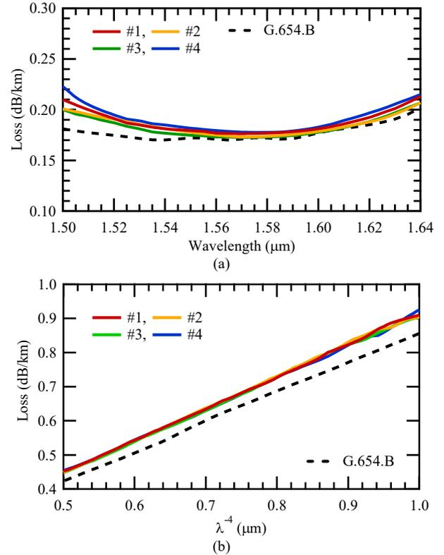
Fig. 4 Measured loss spectrum as a function of (a)  $\lambda$  and (b)  $\lambda^{-4}$
