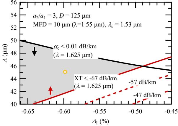
Fig. 2 Calculated values of the inter-core XT and  $\alpha_c$  as functions of  $\Delta_1$  and  $\Delta$
