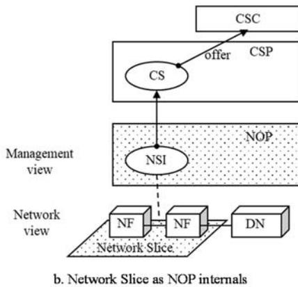
Fig. 6: Service offerings by Network Slice [19].
