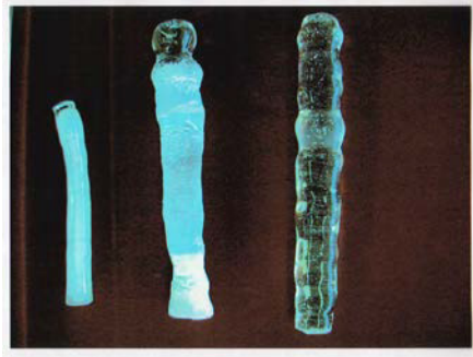
図 3 透明化に失敗した試料 Fig. 3 Failed samples in consolidation process.
