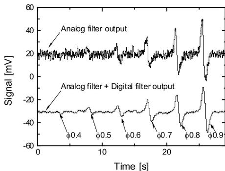
**Fig. 7** Time traces of signals from steel balls with different diameters. The upper section shows the trace prior to the digital filtering process, and the lower section shows the trace after the digital filtering process.
