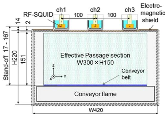
**Fig. 3** Detailed cross-sectional view of the detection region.
