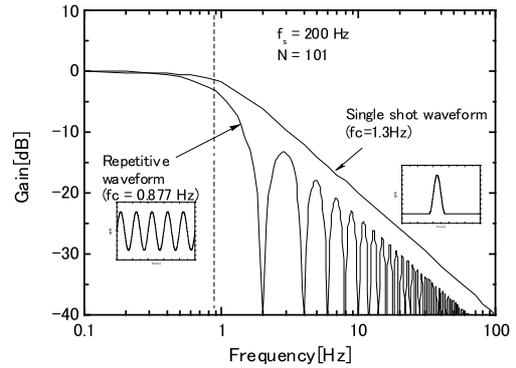
**Fig. 6** Gain characteristic for frequency  $f$  of the digital filter with  $f_s$  of 200 Hz and  $N = 101$  for repetitive waveform. Experimentally measured gain characteristics for single shot waveform is also shown for comparison.
