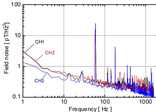
**Fig. 2** Magnetic field noise of the each RF-SQUID.
