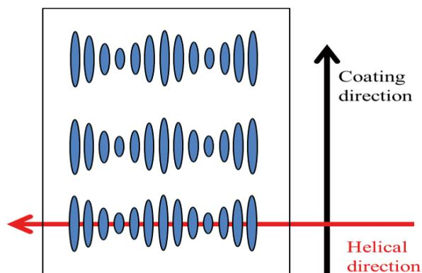
**Fig. 4** Illustrated model of the slit-coating direction and the resultant helical direction
