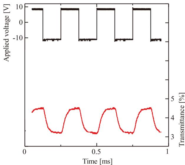
Fig. 6 Electro-optical response of the ULH LCD, where the driving rectangular voltage was  $20 V_{p-p}$ , 4 kHz
