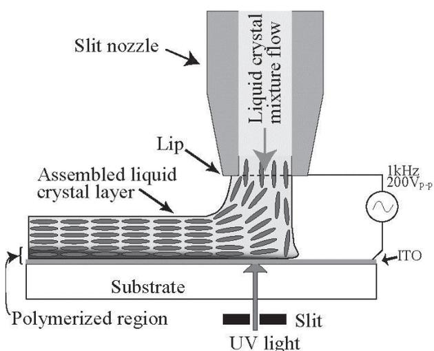
**Fig. 1** Schematic model of the slit coater, where AC voltage as a stabilization of the helix was applied between the slit lips and the ITO electrode
