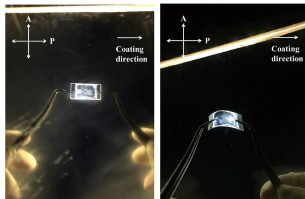
**Fig. 2** Aspects of the ULH LCD where PC films were used as the substrate
