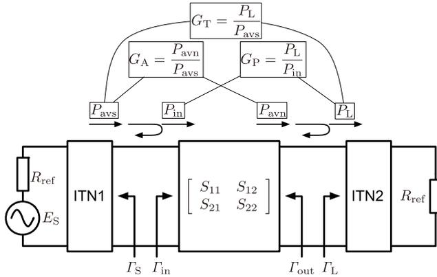
Fig. 15 Power gains of a 2-port.  $\Gamma_{in}$ : Input reflection coefficient.  $\Gamma_{out}$ : Output reflection coefficient.  $P_{avs}$ : Power available from the source.  $P_{in}$ : Power absorbed by the 2-port network.  $P_{avn}$ : Power available from the 2-port network.  $P_{in}$ : Power absorbed by the load. ITN: Impedance transforming network.
