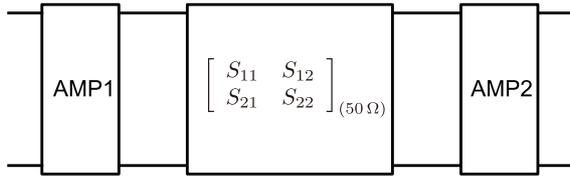
Fig. 14 A single amplifying stage within a multi-stage amplifier.
