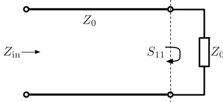
**Fig. 3** A length of transmission line terminated with its characteristic impedance  $Z_0$  at the far end looks as if the line were infinitely long as seen from the near end.  $Z_{in} = Z_0$  and  $S_{11(Z_0)} = 0$ .
