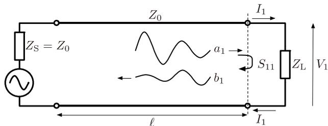
**Fig. 1** A length,  $\ell$ , of transmission line driven by a matched source (source impedance  $Z_S = Z_0$ ) and terminated with a load impedance  $Z_L$ .  $Z_0$  is the characteristic impedance of the line.
