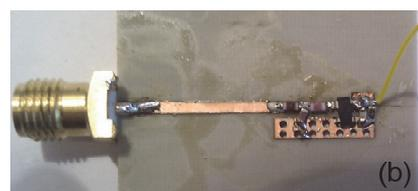
**Fig. 1** Rectifier circuit at 433 MHz. (a) Schematic of the envelope detector rectifier, (b) photo of the prototype.
