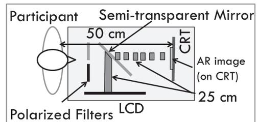
Fig. 7 Arrangement of apparatus for Experiment 2.
