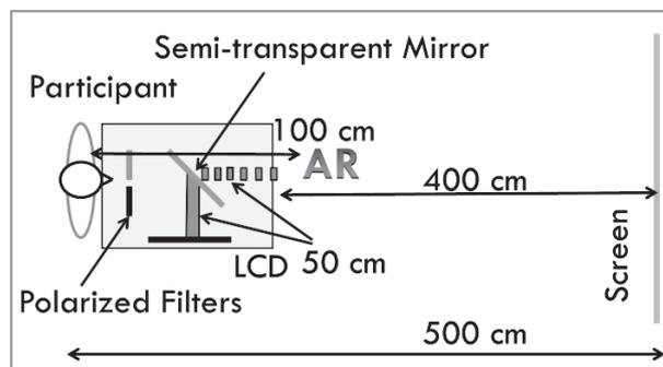
Fig. 1 Arrangement of apparatus for Experiment 1.
