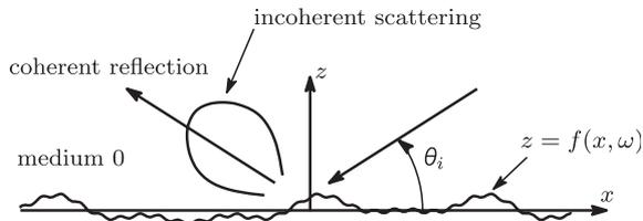
**Fig. 7** Scattering from a homogeneous random surface. The coherent reflection into the specularly reflected direction and incoherent scattering into all directions.
