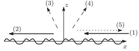
**Fig. 5** Reciprocity. When a plane wave is incident with a low grazing angle from a direction (1), diffraction into directions (3) and (4) disappears. Only the reflected wave propagating into a grazing direction (2) may exist. Furthermore, a plane wave into another grazing direction (5) can exist if the periodic surface satisfies the double anomaly condition.
