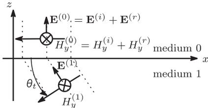
**Fig. 2** Electromagnetic field at low grazing angle of incidence. A dotted line indicates an equi-phase plane.
