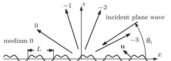
**Fig. 4** Diffraction by a perfectly conductive periodic surface.
