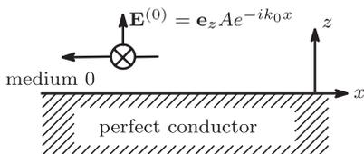
**Fig. 3** A guided wave propagating along a flat surface.
