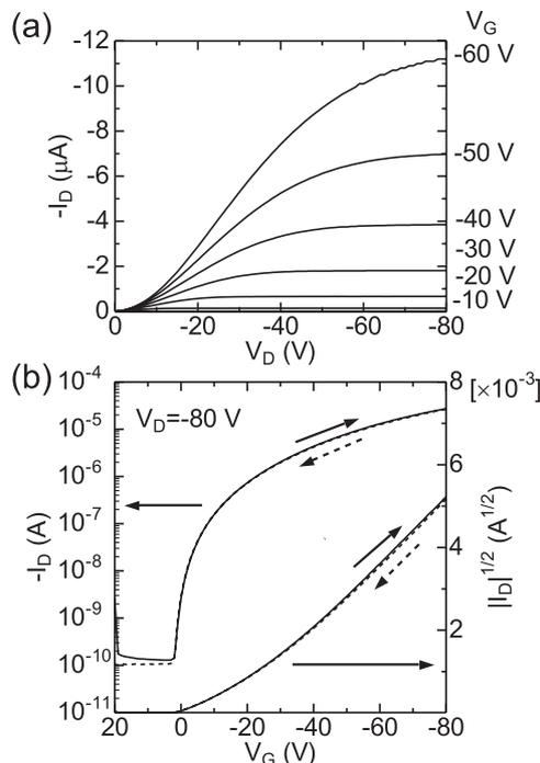
**Fig. 5** (a) Output and (b) transfer characteristics of PBTTT FET with  $L=50\mu\text{m}$  fabricated using the self-aligned method.
