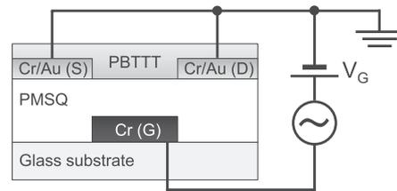
**Fig. 2** Experimental setup for the impedance measurements of OFETs used in this study.
