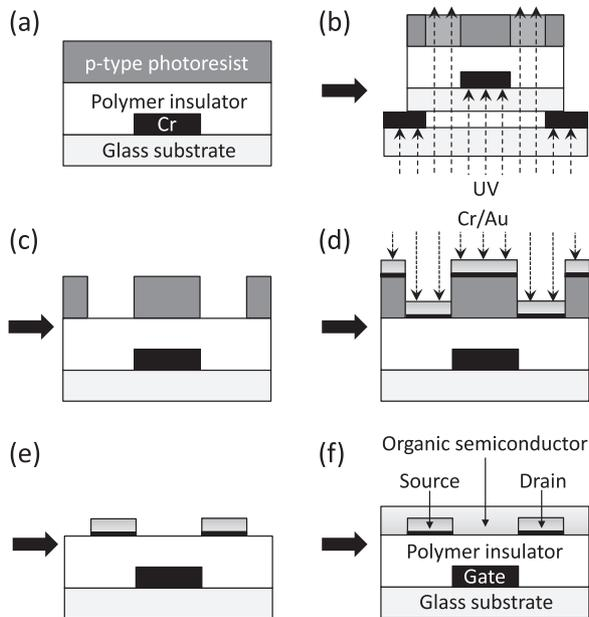
**Fig. 1** Schematics of the fabrication processes of solution-based OFETs with polymer gate insulators using the self-aligned method.
