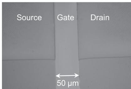
**Fig. 3** Optical microscope image of PBTTT FET with  $L=50\mu\text{m}$  fabricated using the self-aligned method.
