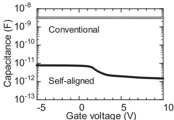
**Fig. 6** Capacitance-gate voltage characteristics of PBTTT FETs fabricated using the self-aligned and conventional methods.
