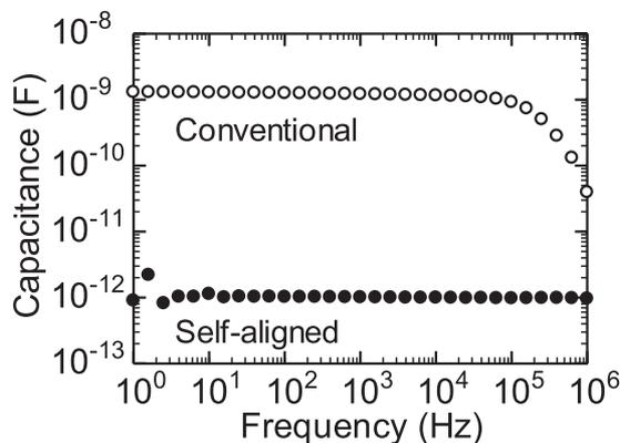
**Fig. 4** Frequency dependence of capacitance between the source-drain electrodes and the gate electrode of electrode configurations fabricated using the self-aligned and conventional methods.
