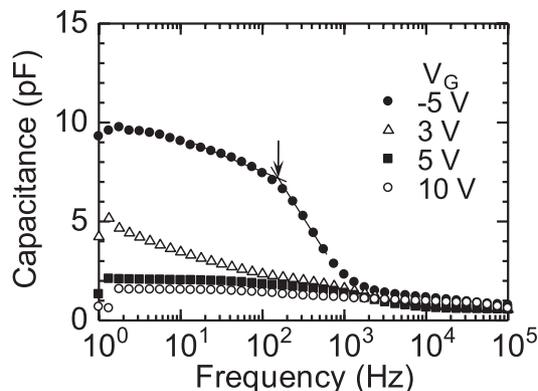
Fig. 7 Capacitance-frequency characteristics measured at different  $V_G$  in PBTFT FET with  $L=50\ \mu\text{m}$  fabricated using the self-aligned method.
