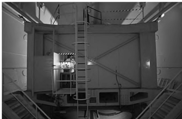
Fig. 7 Capsule located at a depth of 500 meters in the LSBB underground laboratory in which SQUIDs are installed.
