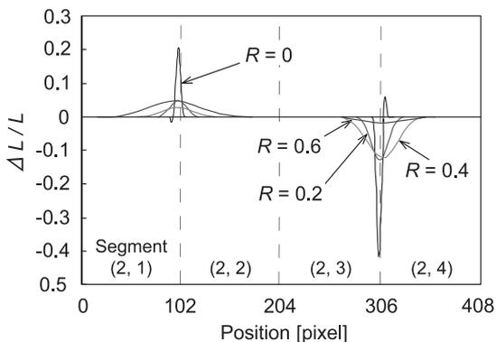
Fig. 9  $\Delta L/L$  vs. position along the horizontal line indicated by the black arrow in Fig. 3(a).
