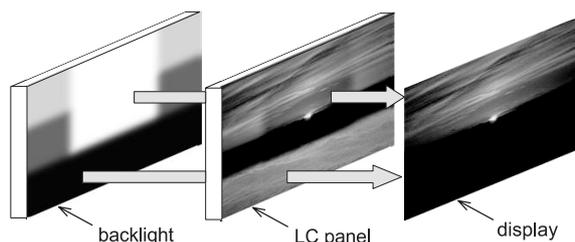
Fig. 1 Principle of the adaptive dimming technique.
