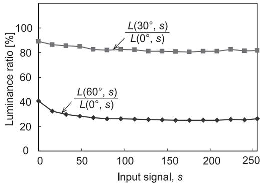
Fig. 6 Luminance vs. TV set input signal for various viewing angles.
