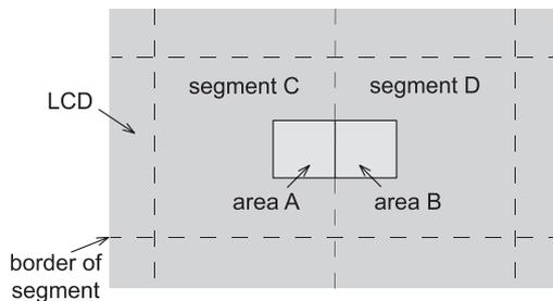
Fig. 4 Example of the adaptive dimming technique. The dimming factors of segment C and D are different but LCD luminance of area A and B is identical.
