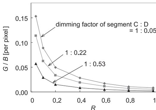
Fig. 10  $G/B$  at the border of the segment as a function of  $R$  for various combinations of the dimming factors of segment C and D in Fig. 4.
