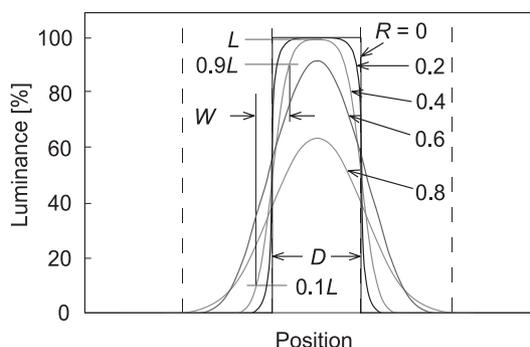
Fig. 8 Cross section of backlight luminance distribution when a segment is fully ignited. As a reference,  $W$  for  $R = 0.4$  is depicted.
