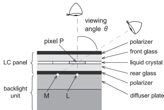
Fig. 5 Principle of image degradation caused by the adaptive dimming technique.
