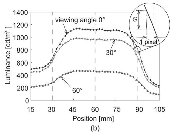
Fig. 7 Backlight luminance distribution along the horizontal direction for various viewing angles. Dimming factors of the segments are (a) same and (b) different.
