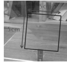
**Fig. 15** The picture of the transparent ITO antenna. The outer dimension of the ITO antenna was 5 cm  $\times$  5 cm.
