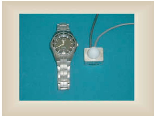
Fig. 7 NRD-guide receiver with lens antenna.
