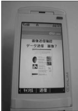
Fig. 3 The thumbnail picture shown on the main display of the mobile phone.
