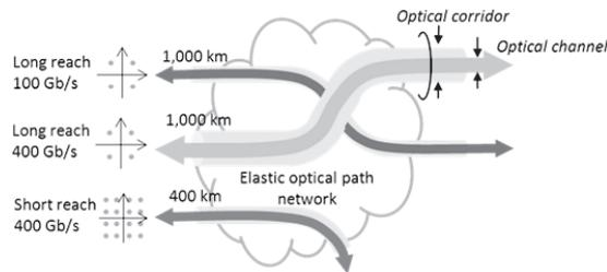
**Fig. 3** Elasticity in optical channels and optical corridors.
