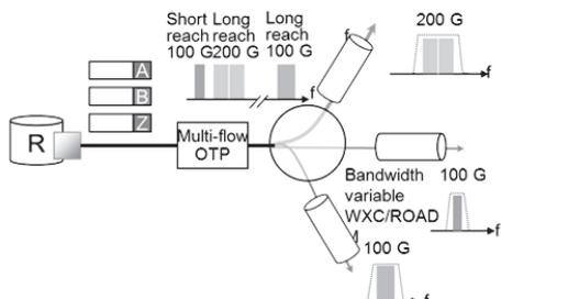
(b) Point-to-multipoint optical connections using multi-flow OTP
