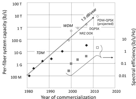
Fig. 2 Trend in per-fiber capacity for transmission systems deployed in Japan.
