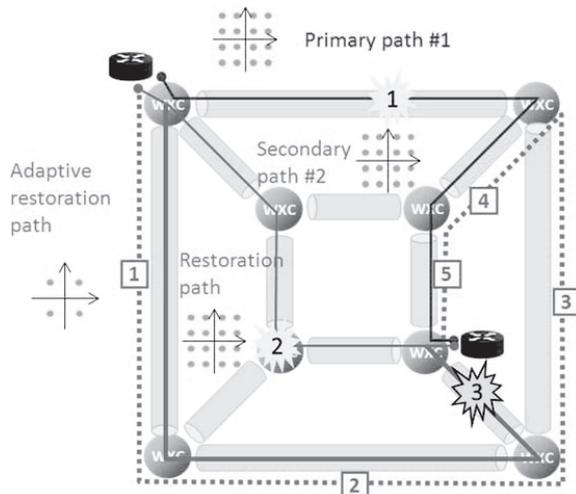
**Fig. 8** Optical layer adaptive restoration.
