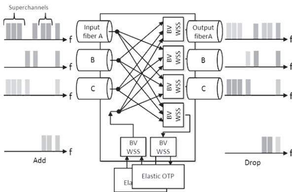
Fig. 4 Possible architecture for a flexible bandwidth WXC.
