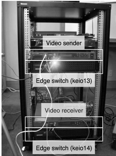
**Fig. 8** High definition video sender, receiver, and 2 edge switches placed in Keio University, Japan.
