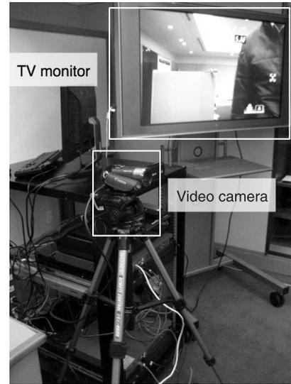
**Fig. 10** High definition video captured by video camera is displayed on TV monitor.
