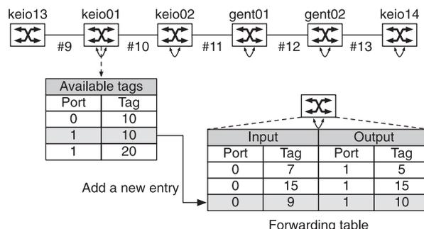
Fig. 7 Changing configurations of a switch when signaling is occurred.
