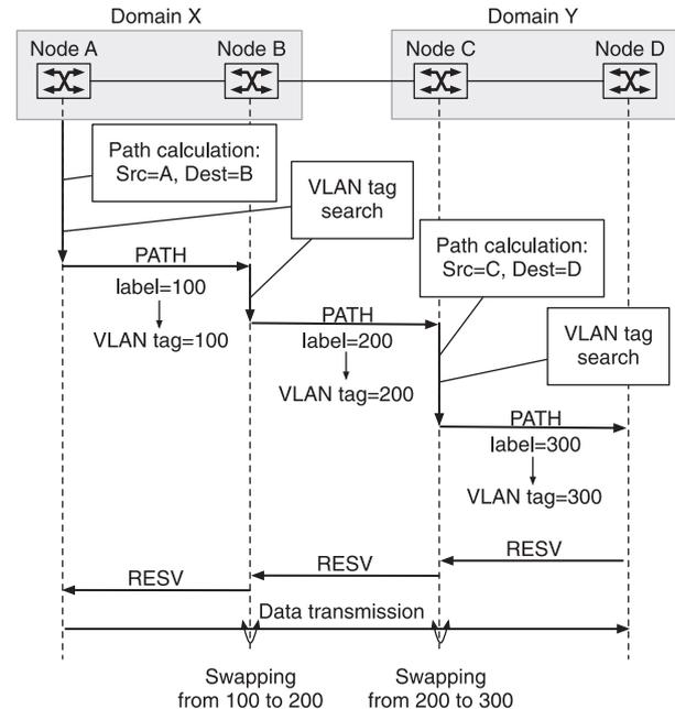
Fig. 4 Signaling sequence of L2-LSP establishment.
