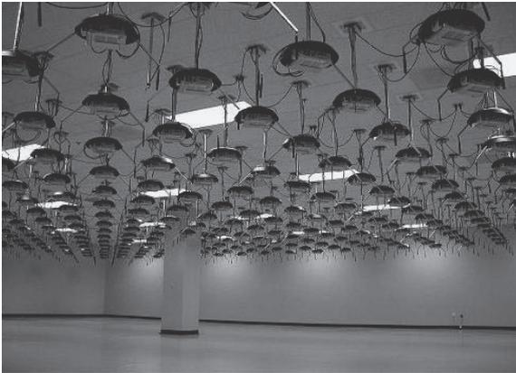
Fig. 6 ORBIT radio grid at WINLAB tech center.
