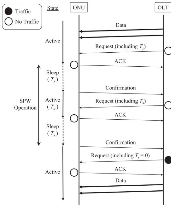
**Fig. 7** SPW operation for downstream traffic.
