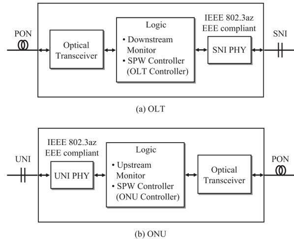
Fig. 4 PON components with power saving functions.
