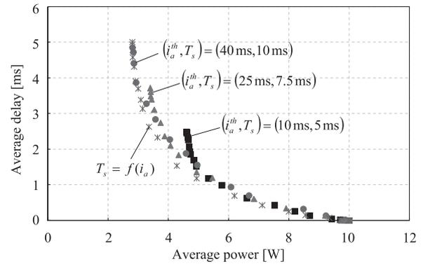
Fig. 14 Relationship between power consumption and queuing delay (variable sleep period).
