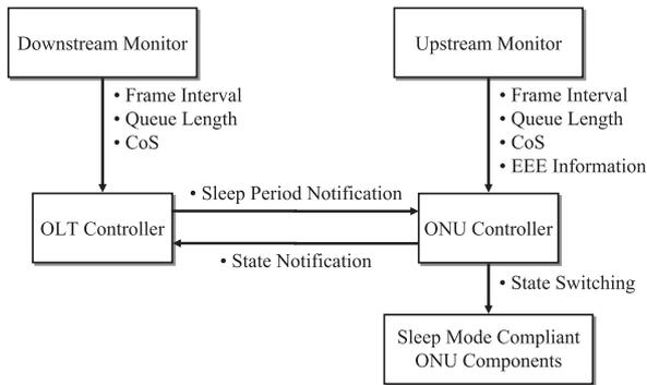
Fig. 5 Block diagram of power saving functions.
