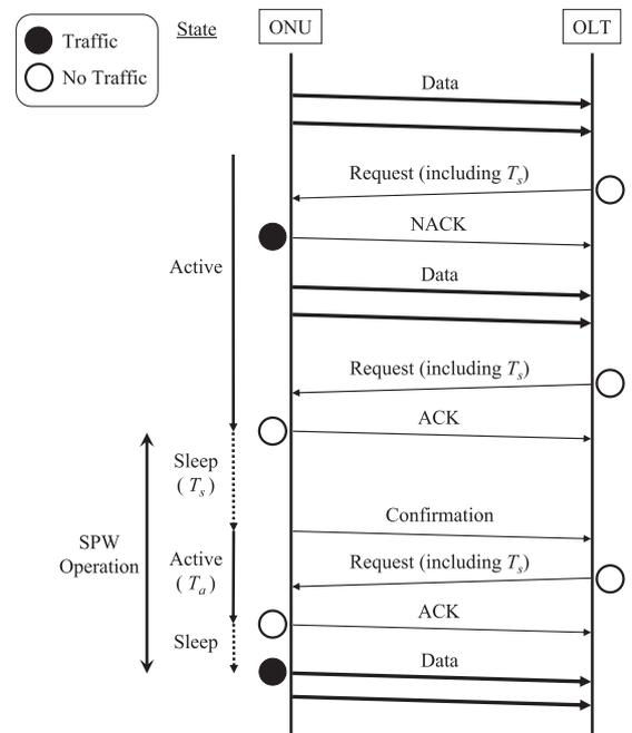
**Fig. 8** SPW operation for upstream traffic.
