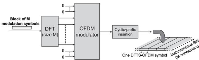
Fig. 1 Basic principle of DFTS-OFDM transmission.
