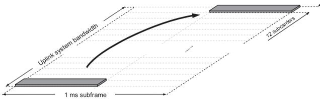
Fig. 3 Uplink control signaling.
