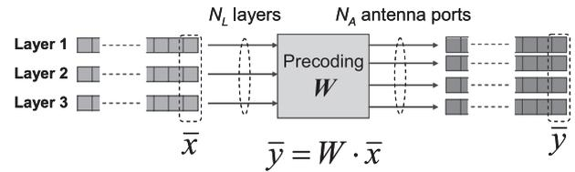
Fig. 5 LTE pre-coder-based spatial multiplexing. Number of layers  $N_L = 3$ .
