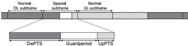
Fig. 4 Frame structure for LTE/TDD.
