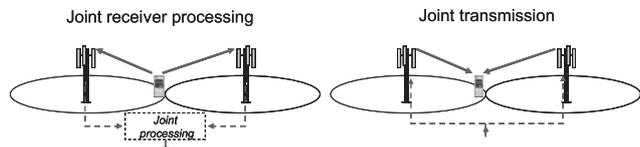
**Fig. 7** Coordinated multipoint transmission/reception based on joint up-link receiver processing and joint downlink transmission, respectively.
