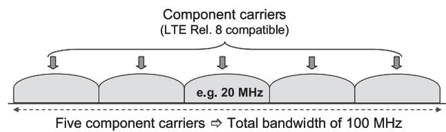
**Fig. 6** Carrier aggregation for extended bandwidth.
