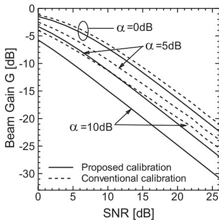
**Fig. 9** Terminal's ZF transmit beam gain  $G$  in direction to  $\mathbf{a}^{(UL)}$  after the conventional calibration or the proposed calibration (allocation 1) with  $T = 1$  and  $\tau = 0.5 \mu\text{s}$ .
