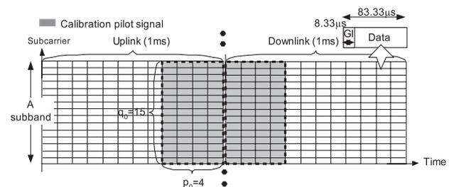
**Fig. 3** Calibration pilot symbols in an OFDMA/TDD system.
