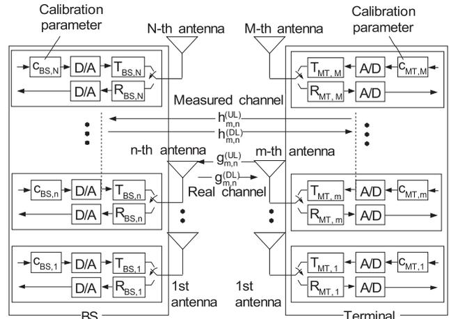
Fig. 1 Signal transmission model in a TDD system.
