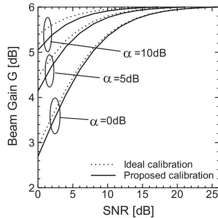
**Fig. 10** Terminal's MRC transmit beam gain  $G$  in direction to  $\mathbf{a}^{(UL)} = [a_{1,1}^{(UL)}, \dots, a_{M,1}^{(UL)}]^T$  after ideal calibration or the proposed calibration (allocation 1) with  $T = 1$  and  $\tau = 0.5 \mu\text{s}$ .
