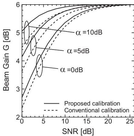
**Fig. 8** Terminal's MRC transmit beam gain  $G$  in direction to  $\mathbf{a}^{(UL)} = [a_{1,1}^{(UL)}, \dots, a_{M,1}^{(UL)}]^T$  after the conventional calibration or the proposed calibration (allocation 1) with  $T = 1$  and  $\tau = 0.5 \mu\text{s}$ .
