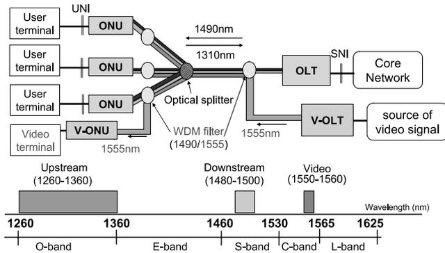
Fig. 2 3-wave multiplexing in B-PON.
