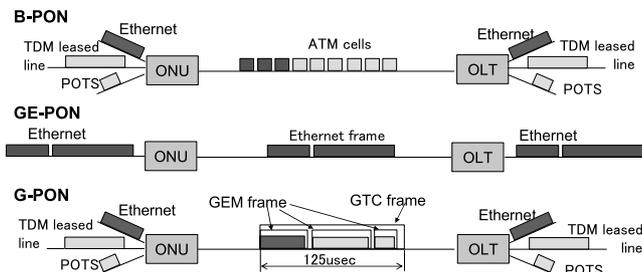
Fig. 10 Frame structures of B/GE/G-PON.
