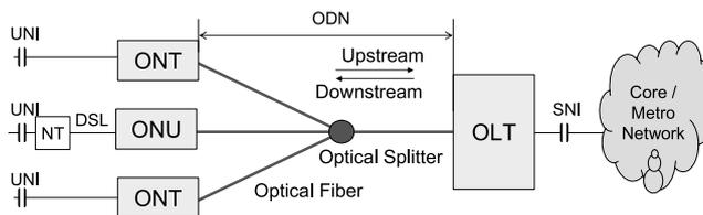
Fig. 1 Schematic of PON configuration.
