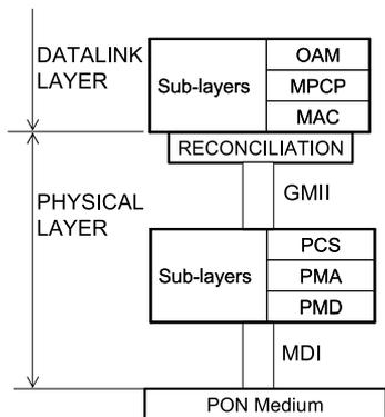
Fig. 4 Layer architecture of GE-PON.
