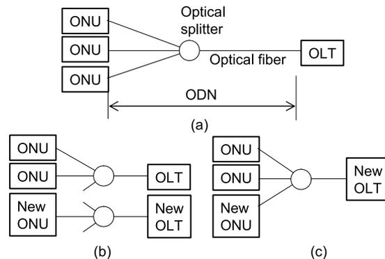
Fig. 11 Schematic view of PON. (a) single system, (b) upgrade without co-existence, (c) upgrade with co-existence.
