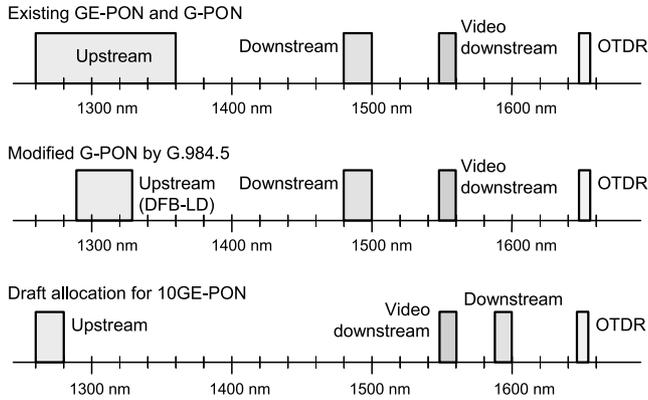
Fig. 12 Draft of wavelength allocation for 10GE-PON.
