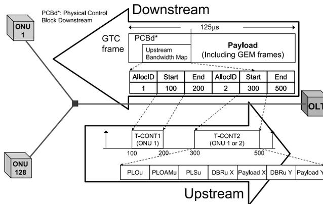
Fig. 6 GTC frame of G-PON.
