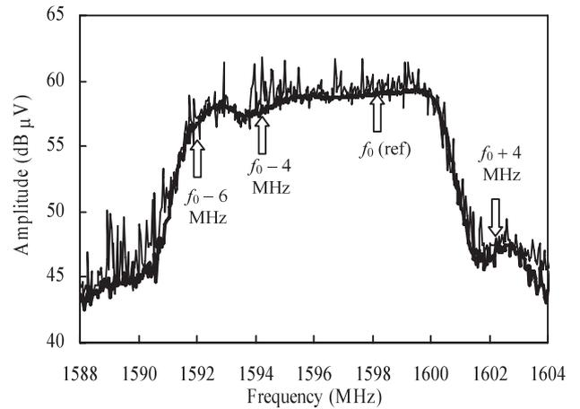
**Fig. 11** Measured spectrum of a wideband disturbance from PC#2 (a harmonic of bus clock with FM). Resolution bandwidth: 1 MHz, peak detection mode. Thick curve indicates averaged spectrum.
