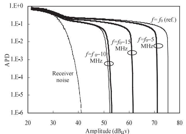
**Fig. 8** Measured (thin lines) and converted (thick lines) APDs of repetitive wideband pulses. Measured APD at  $f = f_0$  was used as reference. Pulse duration:  $0.1 \mu\text{s}$ , repetition frequency: 100 kHz, and resolution bandwidth: 1 MHz.
