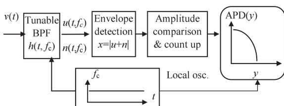
Fig. 1 Schematic diagrams of APD measuring receiver.
