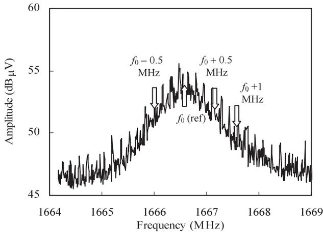
**Fig. 9** Measured spectrum of a narrowband disturbance from PC#1 (clock harmonic without FM). Resolution bandwidth: 1 MHz, peak detection mode.
