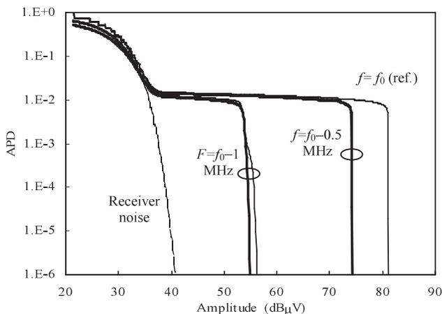
**Fig. 6** Measured (thin lines) and converted (thick lines) APDs of repetitive narrowband pulses. Measured APD at  $f = f_0$  was used as reference. Pulse duration:  $10 \mu\text{s}$ , filtered by Gaussian BPF ( $B = 0.3 \text{ MHz}$ ), repetition frequency: 1 kHz. Resolution bandwidth: 1 MHz.
