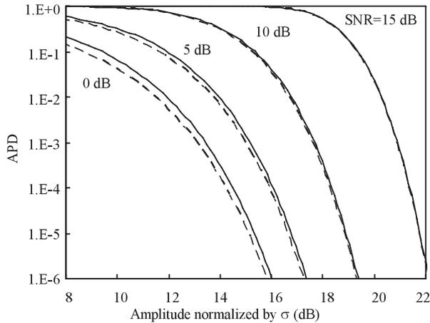
**Fig. 3** Comparison of APDs of Rice distribution (solid lines) and approximation by Gauss distribution (broken lines) for various SNRs.
