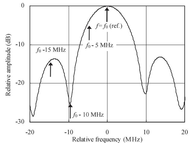
**Fig. 7** Measured spectrum of a train of repetitive wideband pulses. Disturbance pulse duration:  $0.1 \mu\text{s}$ , repetition frequency: 100 kHz. Resolution bandwidth: 1 MHz.
