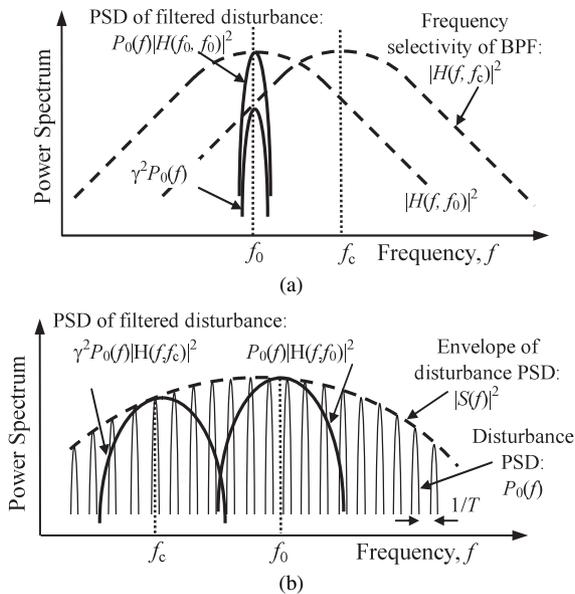
**Fig. 4** Estimating scale factor  $\gamma$ . (a) Narrowband disturbance:  $\gamma^2 = |H(f_0, f_c)/H(f_0, f_0)|^2$  (b) Wideband pulsed disturbance:  $\gamma^2 = |S(f_c)/S(f_0)|^2$
