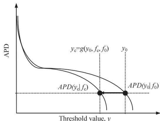
Fig. 2 Schematic illustration of conversion of a disturbance APD from a frequency  $f = f_0$  to  $f = f_c$ .
