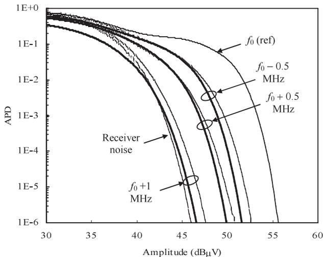
**Fig. 10** Measured (thin lines) and converted (thick lines) APDs of narrowband disturbance from PC#1 (spectrum is shown by Fig. 9). Measured APD at  $f = f_0$  was used as reference. Resolution bandwidth: 1 MHz.
