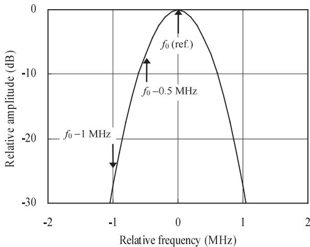
**Fig. 5** Frequency selectivity of APD measuring receiver. Impulse bandwidth = 1 MHz, Gaussian filter.
