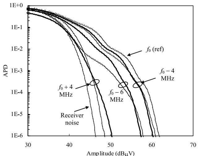
**Fig. 12** Measured (thin lines) and converted (thick lines) APDs of wideband disturbance from PC#2 (the spectrum is shown by Fig. 11). Measured APD at  $f = f_0$  was used as reference. Resolution bandwidth: 1 MHz.
