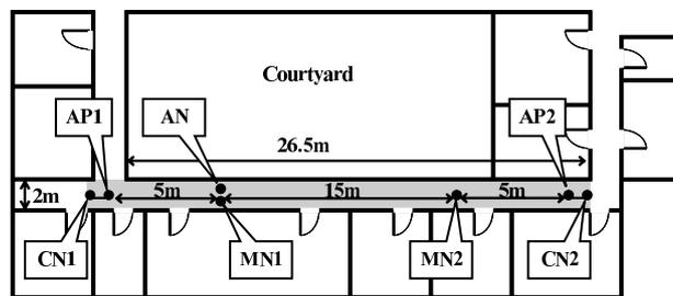
Fig. 9 Experimental environment for evaluating the effect of radio interference.
