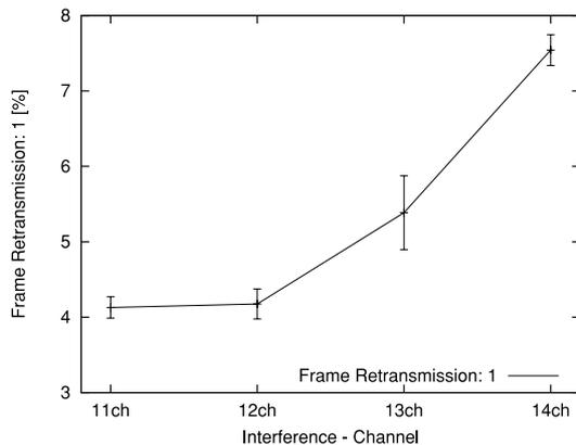
Fig. 12 Frame retransmission ratio under radio interference.
