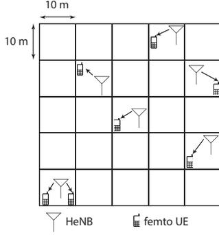
**Fig. 2** Femtocell deployment in 5 x 5 grid model.
